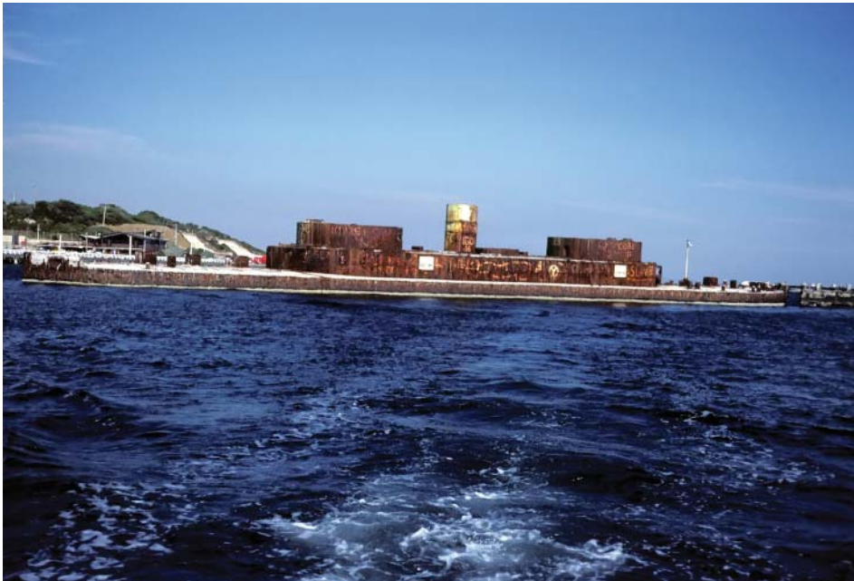
FIGURE 3 View of HMVS Cerberus in 1977 showing original profile and the relatively low free board.
