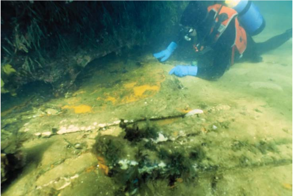
FIGURE 5 Diver inspecting the active corrosion on detached hull plates as shown by the red-brown colouration October 1994.
